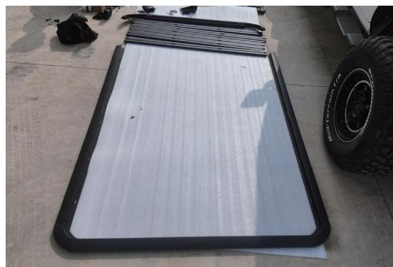
Prepare the required part (②\*1). As shown in the diagram, Remove the pre-installed screws from ②. Connect the pre-assembled ⑤ to ②. Secure the connection using the removed screws.
