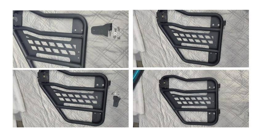
Prepare required components (1\*1, 3\*1, 4\*1, b\*4, c\*4, e\*4), Connect 1 to 3 with b, c, e, then connect 1 to 4 with b, c, e. (Note: do not tighten screws completely, 3 and 4 have different thread lengths)
