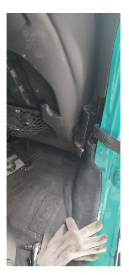
Prepare required components (d\*2) ,as shown in the diagram, secure the hinge with d, and fix the limiter strap inside the vehicle.
