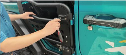
Mount the door to the vehicle body, close the door, then fully tighten the screws.
