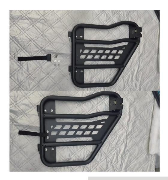
Prepare required components (2\*1, a\*2, b\*2, c\*2), as shown in the diagram,install 2 to the car door using a,b, c.
