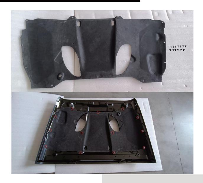
Prepare the required parts (2\*1, a\*13). As shown in the diagram, secure component 2 to the hood using a at the red-circled holes..
