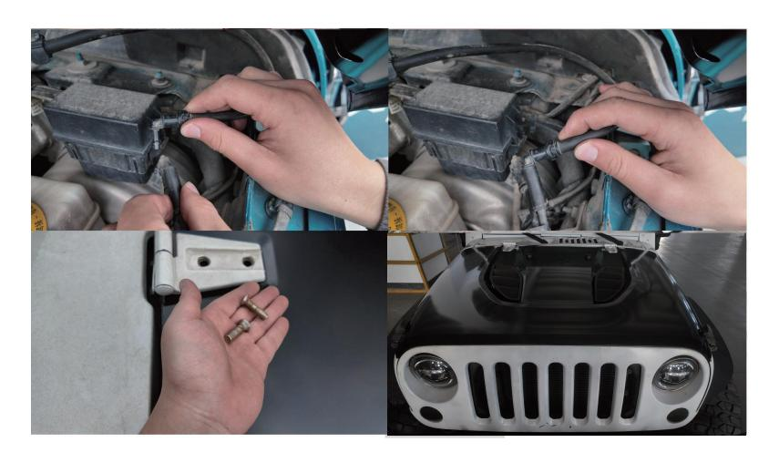
Position the hood onto the vehicle body, connect the coolant hose, and secure the hinges to the hood using the OEM screws.
