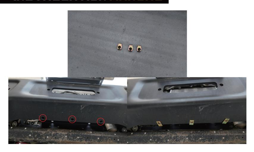
Prepare the required parts (d\*3). As shown in the diagram, install d at the red-circled holes.
