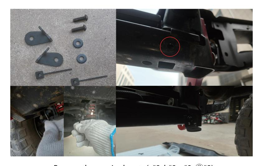
Prepare the required parts (a\*2, b\*2, e\*2, 2\*2). As shown in the diagram, secure 2 to the frame rails using a, b, and e at the red-circled holes. (Note: Adjust the state of e manually to align with the holes.)
