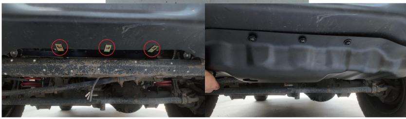
Prepare the required parts (a\*3, b\*3, 1\*1). As shown in the diagram, connect 1 to the bumper using a and b at the red-circled holes.
